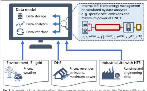
**Fig. 3** Schematics of the data model with the connected systems and its acquired data. Necessary KPI can be accessed by an advanced energy management or are being processed within the data analytics
