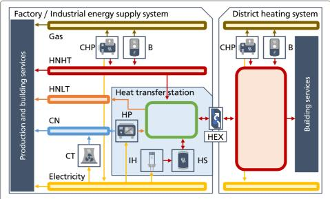
**Fig. 1** Industrial heat transfer station as an autonomous subsystem of an industrial energy supply system, flexibly connecting the industrial site with the district heating system
