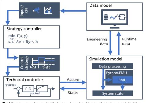
**Fig. 4** Two stage control approach of the heat transfer station with connection to the data and simulation model. The simulation model is integrated as a functional mock-up unit
