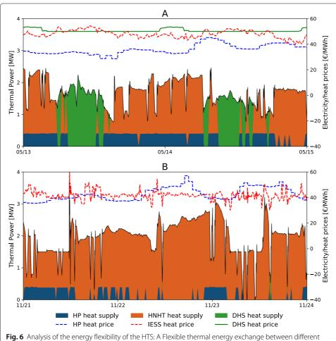
**Fig. 6** Analysis of the energy flexibility of the HTS: A Flexible thermal energy exchange between different heating networks, B Power to heat flexibility
