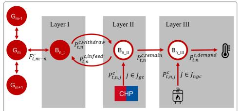
**Fig. 2** Each building or central conversion node n is modeled with three layers. Layer I represents the grid connection of node n, balancing withdrawal and infeed with the edge flows. Layer II considers the output from conversion units, which can feed their output into the grid, while layer III considers the output of all remaining units, the exogeneous energy demand and the input into all technologies in node n
