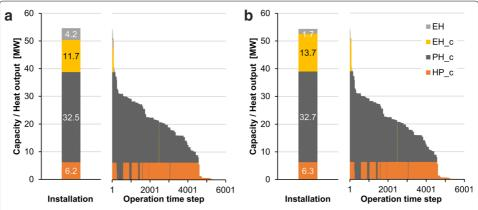
**Fig. 4** Installed capacities and operation duration curves of heating units within the entire system. Central heat pumps (HP\_c) and central pellet heaters (PH\_c) provide base load, central and decentral electric heaters (EH\_c and EH, respectively) provide peak load
