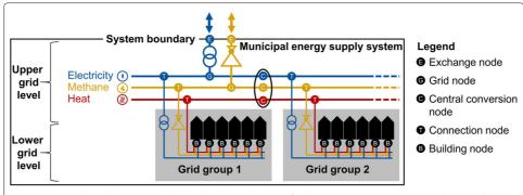
Fig. 1 The grid model contains individual nodes and edges for the energy carriers electricity, heat, and gas. 'Building nodes' and 'central conversion nodes' span across all energy carriers and connect these. The grid of each energy carrier consists of the 'upper' and 'lower' grid level connected at 'connection nodes'
