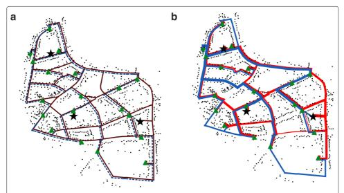
**Fig. 3** (a) Overview of test case with 900 buildings (black dots) in 18 grid groups with central conversion nodes (stars), connection nodes (green upwards triangles), and exchange nodes (green downwards triangles). Possible electric (blue) and heat (red) grid connections on the upper grid level. (b) Expansion result of electric and heat grid on upper grid level
