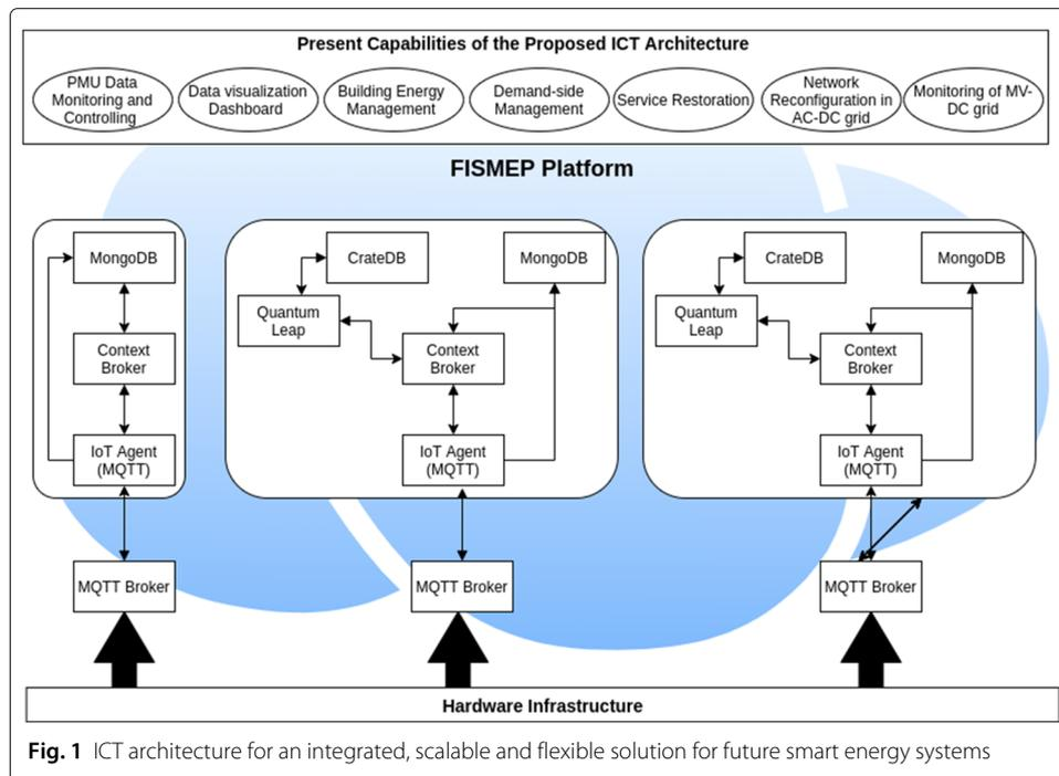
**Fig. 1** ICT architecture for an integrated, scalable and flexible solution for future smart energy systems
