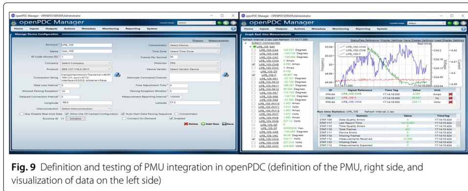
**Fig. 9** Definition and testing of PMU integration in openPDC (definition of the PMU, right side, and visualization of data on the left side)
