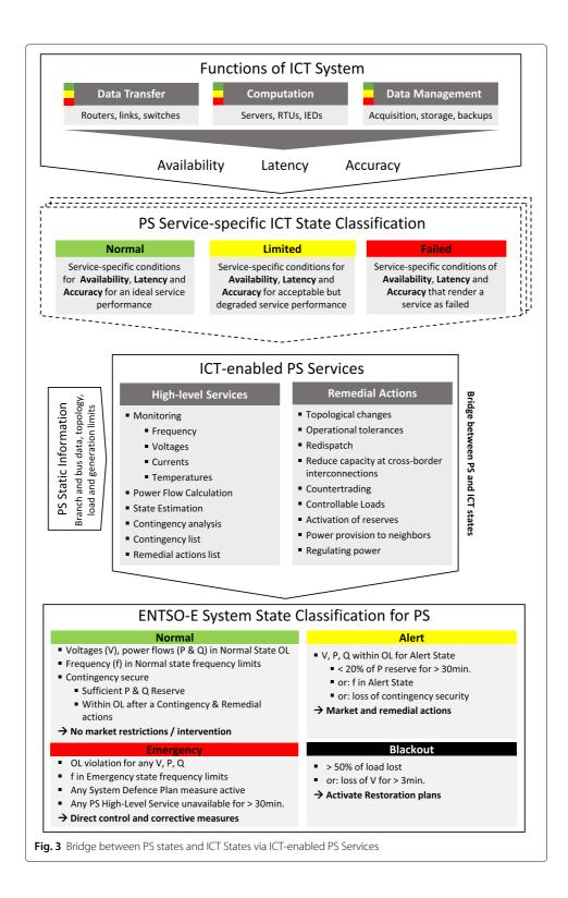
it. In this paper, ICT systems includes field devices, communication network as well as the processing devices such as servers. The operational state in this paper considers both the ICT infrastructure as well as the performance of the grid services it enables.
