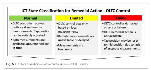
back mechanism as shown in case study 2, i.e., operation based on local measurement. This is referred to as the Limited state of the OLTC service. The Limited and the Failed states of OLTC service are similar to that of case study 2 and are shown in Fig. 6.
