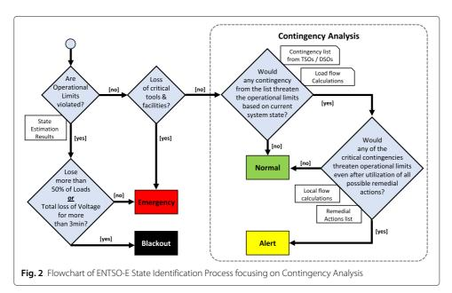
lation yet. Another condition that triggers the Alert State is a lack of more than 20% of the required amount of active power reserves for more than 30 min.
