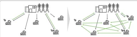
**Fig. 1** The electricity market is experiencing a shift to more distributed energy generation and an increasing share of prosumers supplying their own energy
