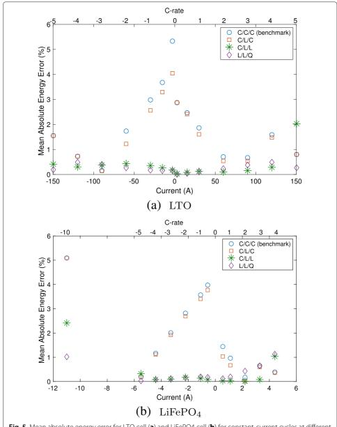
Fig. 5 Mean absolute energy error for LTO cell (a) and LiFePO4 cell (b) for constant-current cycles at different C-rates (top scale)/Amperes (bottom scale)
