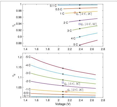
**Fig. 4** The charging and discharging efficiencies of an LTO cell with  $R_{ic} = R_{id} = 0.002~m\Omega$ . Each solid line represents the efficiency calculated using Eqs. 7 or 8 at the labeled charging/discharging C-rate. Each asterisk represents the approximation where  $V = V_{nom,c}$  for charging and  $V_{nom,d}$  for discharging. The constant approximations  $\bar{\eta_c}$  and  $\bar{\eta_d}$  are shown for two labeled operating ranges
