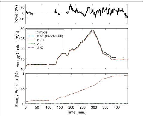
**Fig. 6** The energy content over 8 hours in a realistic deployment charge/discharge profile. The residual between the analytic models and the PI model (bottom), as well as the applied power trace (top), are also shown
