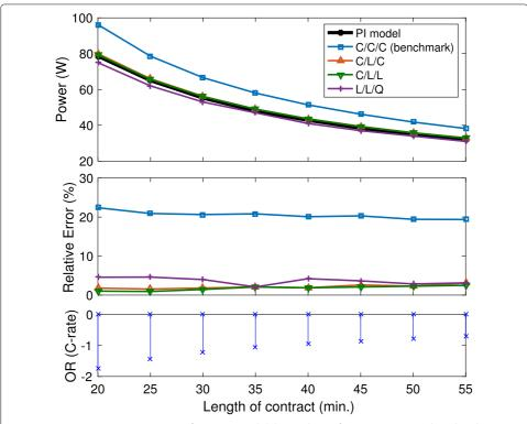
**Fig. 9** Maximum power commitment for guaranteed delivery, shown for various contract lengths. The relative error with respect to the PI model is also shown. The OR figure shows the actual OR determined from the PI model simulation
