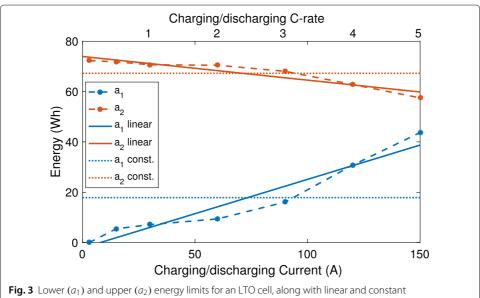
**Fig. 3** Lower  $(a_1)$  and upper  $(a_2)$  energy limits for an LTO cell, along with linear and constant approximations computed over the maximum OR of the battery (up to 5 C charging and discharging)
