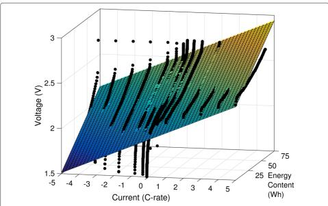
**Fig. 2** *M* function, represented by the black dots which map the applied current and energy content to a unique voltage and are obtained from a spec sheet. The plane is a linear approximation to the *M* function (Eq. 14)
