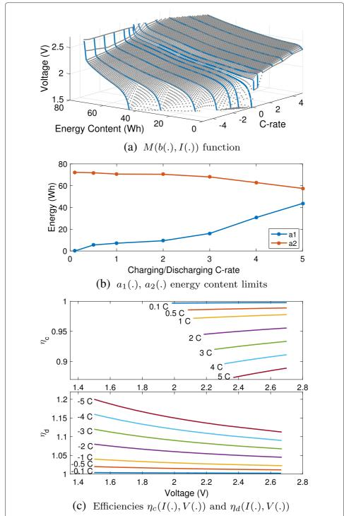
**Fig. 1 a** M function, which maps the applied current and energy content to a unique voltage, shown with blue curves obtained from a spec and grey points representing the interpolated surface between the curves. **b**  $a_1(.)$  and  $a_2(.)$ : points obtained from the spec. **c**  $\eta_c(.)$  and  $\eta_d(.)$ , with each line representing the efficiency at a different C-rate, as per Eqs. 7 and 8
