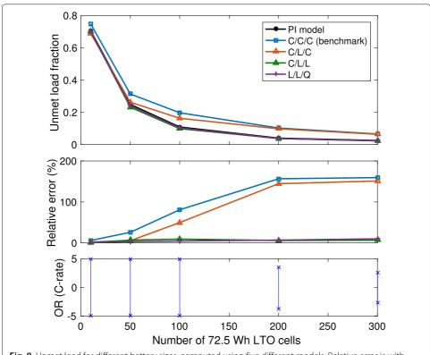
Fig. 8 Unmet load for different battery sizes, computed using five different models. Relative error is with respect to the PI Model, and the effective OR calculated by the PI model is shown in the bottom-most figure
