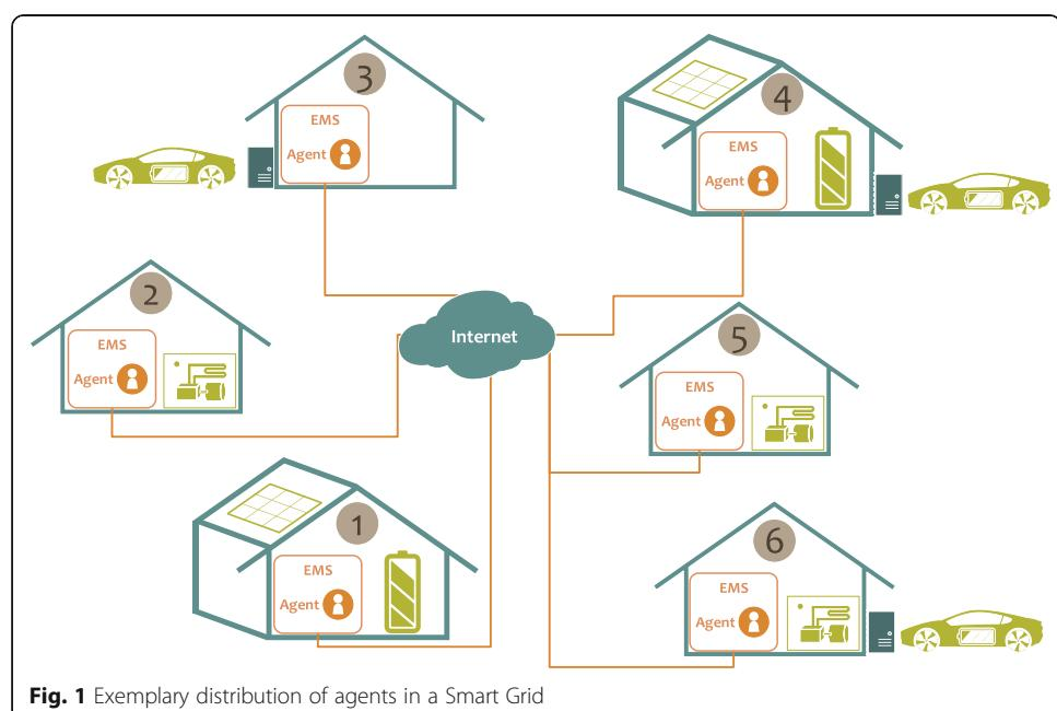
The location of the agents in a central facility revokes some of the major benefits of the distributed algorithm: The robustness of the system is reduced through the reintroduction of a single point of failure. Furthermore the scalability is decreased.
