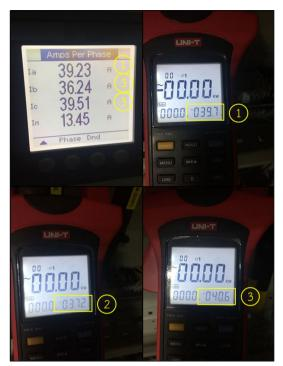
Fig. 4 Comparison of installed meter values and clamp reading
