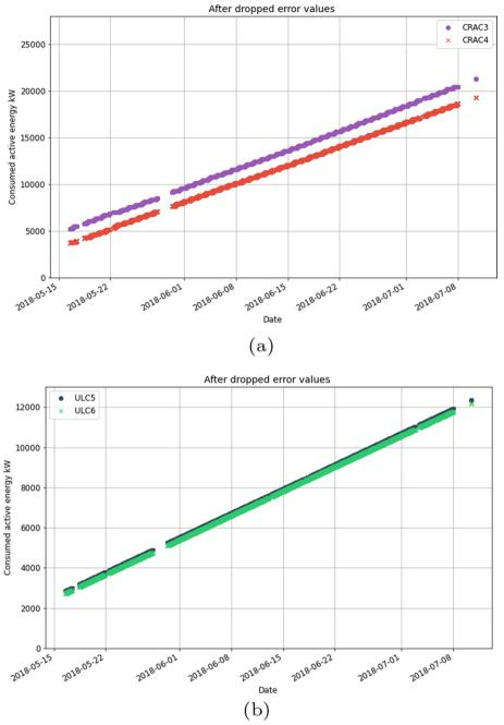
Fig. 11 Consumed active power (drop values) a CRAC3 and CRAC4 b ULC5 and ULC6
