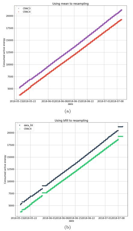
Fig. 12 CRAC3 and CRAC4 consumed active power a mean b bfill
