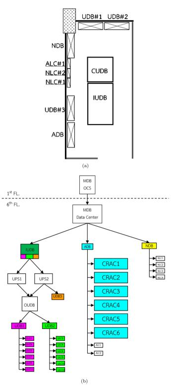
Fig. 2 a Floor plan of the main electricity room (MDB) b Meter connection layout
