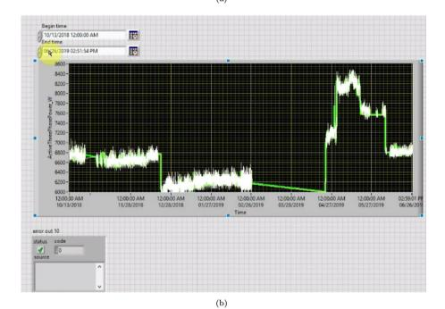
Fig. 24 Labview program UI a Calculation of billing cost based on active power b Moving average of active power
