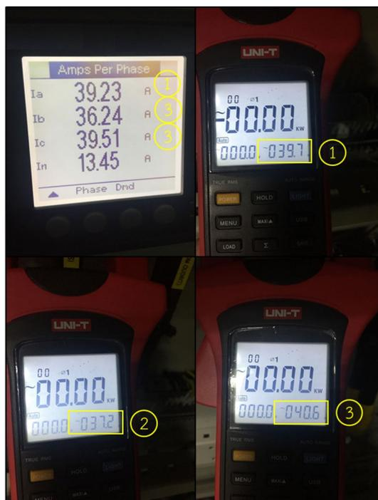
**Fig. 4** Comparison of installed meter values and clamp reading
