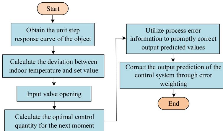
Fig. 6 Flowchart of optimization model for output temperature control based on DMC algorithm
