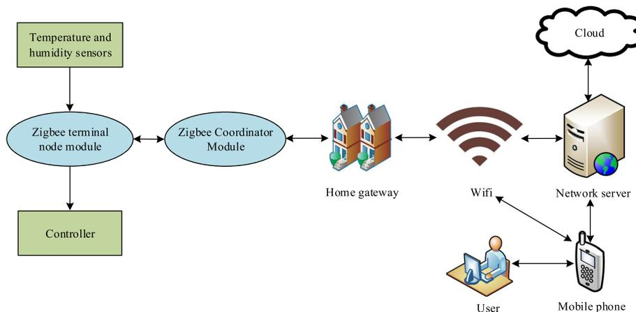
**Fig. 4** The overall structure diagram of the intelligent heating system
