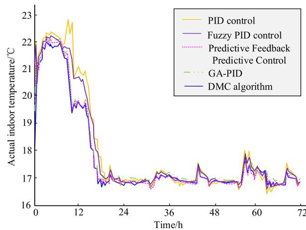
**Fig. 13** Five methods for controlling indoor temperature
