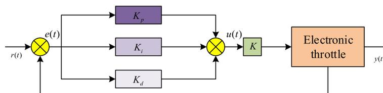
Fig. 5 Structural diagram of PID control strategy
