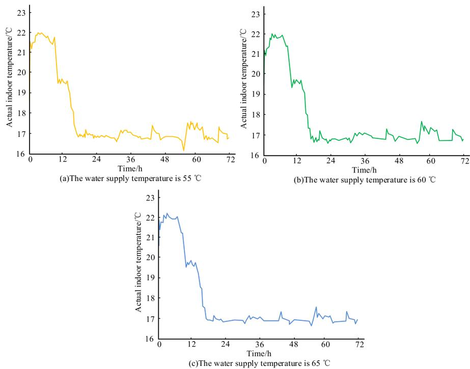
**Fig. 12** The temperature control effect of the model under different water supply temperatures
