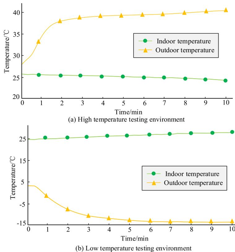
Fig. 10 Test results in high and low temperature environments
