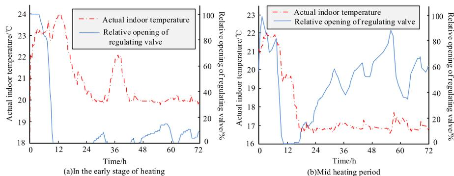
**Fig. 11** The variation of actual indoor temperature and relative opening of regulating valves over time
