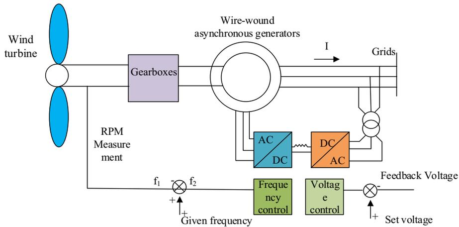
**Fig. 1** Model of wind turbine power generation equipment
