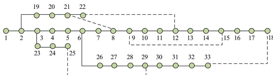
**Fig. 3** IEEE-33 bus distribution node system
