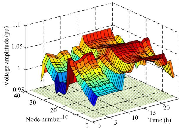
**Fig. 8** 24-h distribution network voltage at each node
