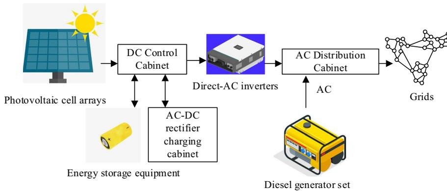
**Fig. 2** Model of solar power generation equipment
