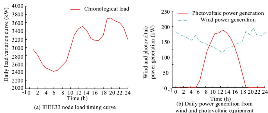
**Fig. 6** 24-h load curve and active output curve
