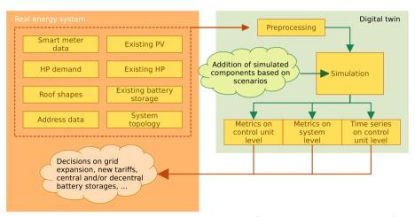
Fig. 4 Required data used by the digital twin and conceptual data flow including the input and output for the simulation
