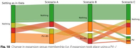
PV-battery-installation or not) for the different evaluated scenarios. The different trajectories are colored differently. We can see that the selected control units for adding components changes significantly depending on the scenario. Scenario D and Scenario E are not shown for the sake of clarity
