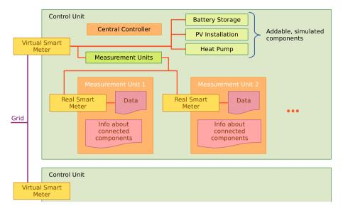
Fig. 2 Concept of a virtual smart meter: Distinction of measurement units as smart meter data input and control units that combine all smart meters in one house and potentially add simulated components. Red lines depict control unit internal energy flows. Crimson lines represent the local energy system
