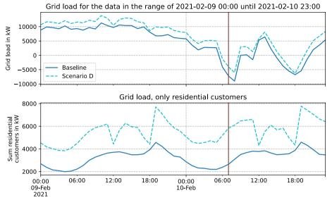
**Fig. 12** Effect of the heat pumps (Scenario D) on grid load for two exemplary days in winter of 2021. The vertical line is placed at 9<sup>th</sup> February 2021, 07:00. Top: Gird load in hourly resolution. Bottom: Grid load without wind farms and large enterprises, i.e. only residential buildings
