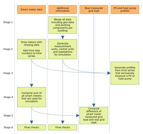
Fig. 7 Overview of the preprocessing pipeline. The orange boxes in the top line depict the different classes of input or output data - i.e., smart meter data from residential households, additional information about addresses, connected components, roof areas etc. of these households, the real measured grid load and PV or heat pump profiles. Green boxes represent processing steps
