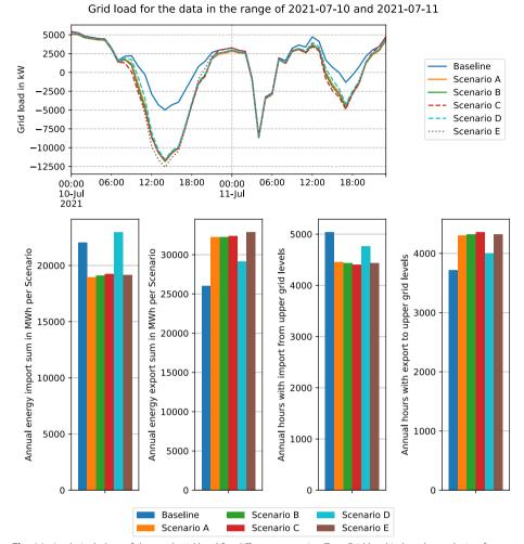
**Fig. 11** Analytical plots of the total grid load for different scenarios. Top: Grid load in hourly resolution for two exemplary days with data taken between 10<sup>th</sup> until 12<sup>th</sup> of July 2021. Bottom: The four graphs show the annual electricity import sum from and export (i.e. feed-in) sum to the upper system level in MWh besides the hours with import from or feed-in to the upper system level per Scenario
