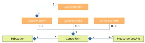
Fig. 6 The UML class diagram of the implementation with the cardinalities given. Orange boxes depict simulated components, green boxes depict units representing real objects
