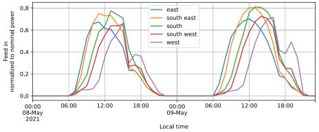
Fig. 8 Plot of exemplary feed-in time series per roof orientation for two days in May 2021
