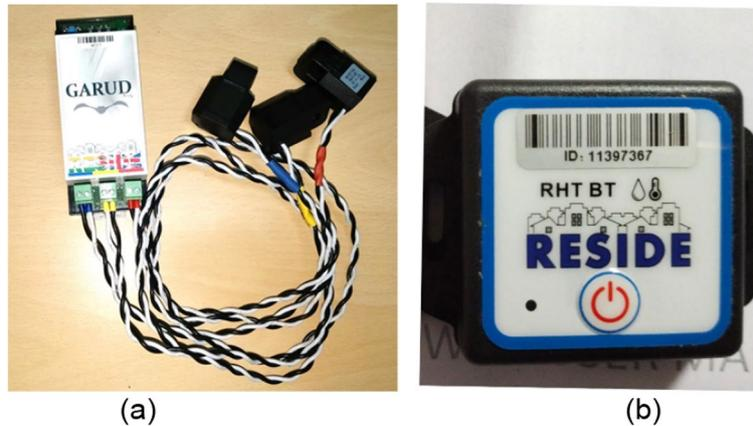
**Fig. 2** Garud and EnviLog loggers used to capture data
