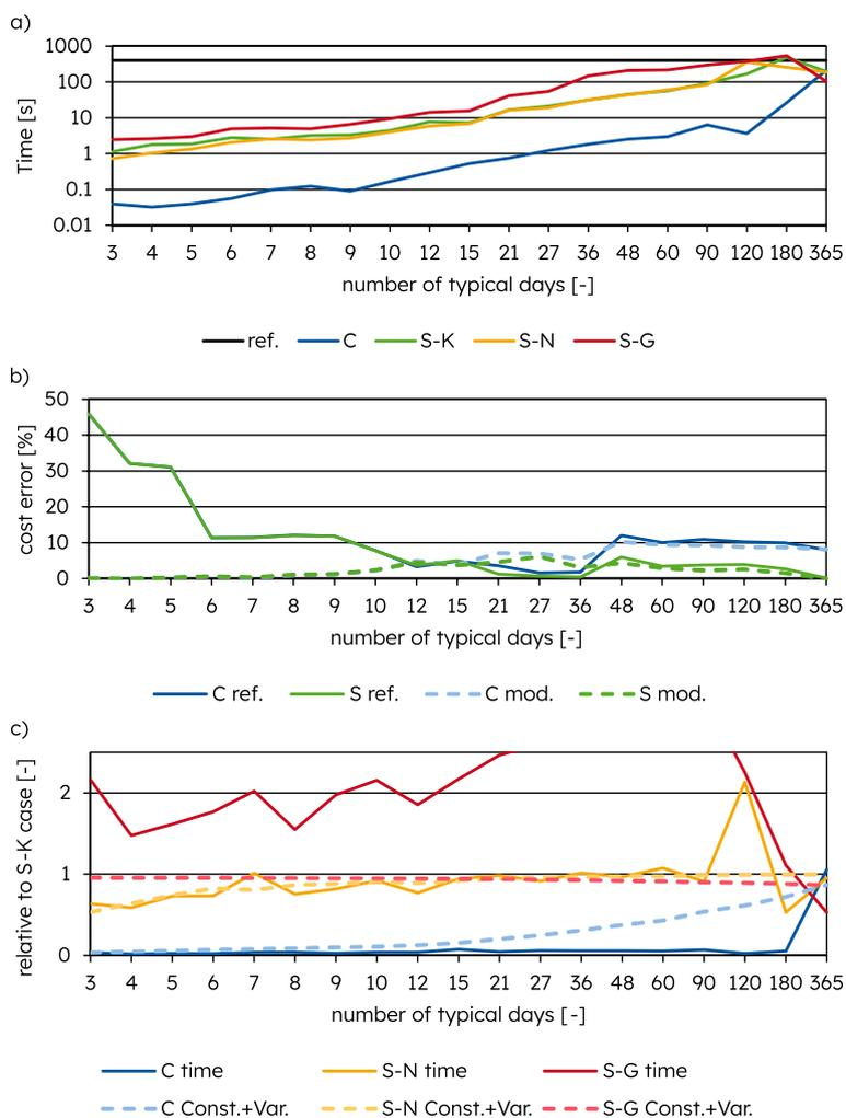
**Fig. 5** Calculation time (a) and total costs error (b) for the different storage models and relative share of number of constraints and variables as well as time for C, S-G- and S-N- to S-K-model (c) for Island system
