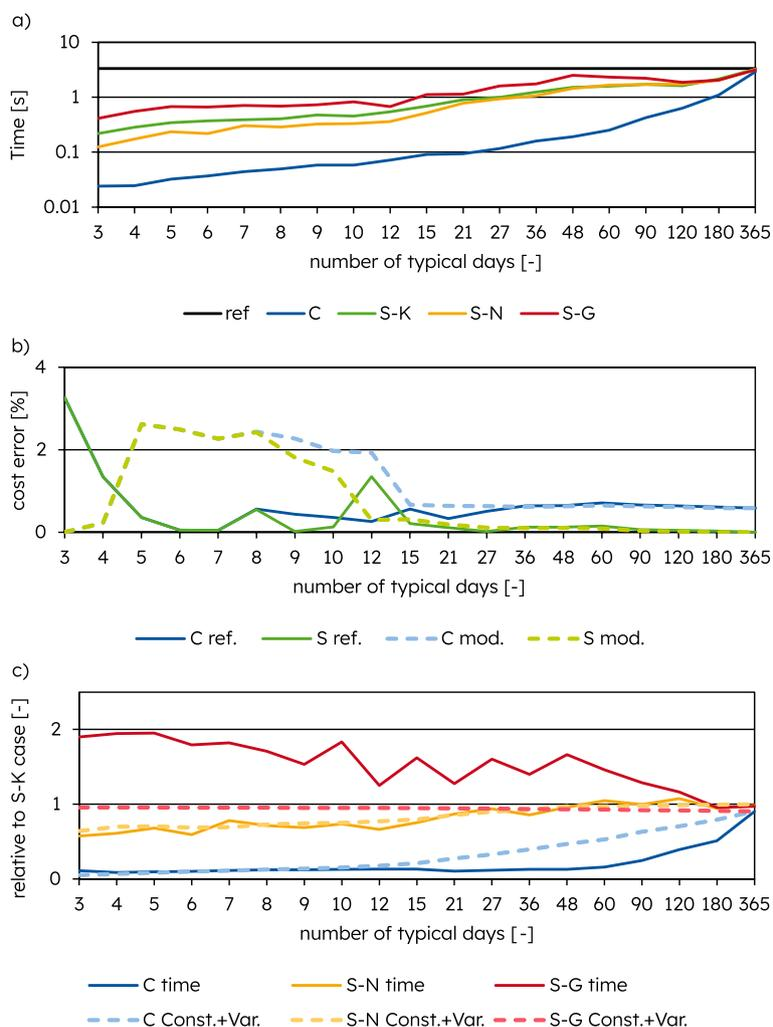
**Fig. 3** Calculation time (a) and total costs error (b) for the different storage models and relative share of number of constraints and variables as well as time for C, S-G- and S-N- to S-K-model (c) for the CHP system
