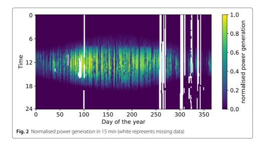
The power output of the tested PV system has been collected at the digital, calibrated energy meter and is averaged to 1 hour mean values for the year 2020 to match the temporal resolution of the ERA5 reanalysis data. Due to some measurement issues, 374 hours are missing and have been excluded from the optimisation. The measured power output and data gaps are visualised with a quarter hourly resolution in Fig. 2.
