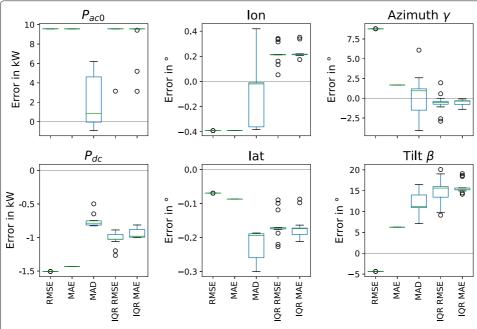
**Fig. 6** Mismatch between the estimated and actual parameters (15 repetitions). Parameters search space according to Table 3. Inverter peak power  $P_{ac0}$  is mostly optimised to the search space boundary, the remaining parameters are within the search space
