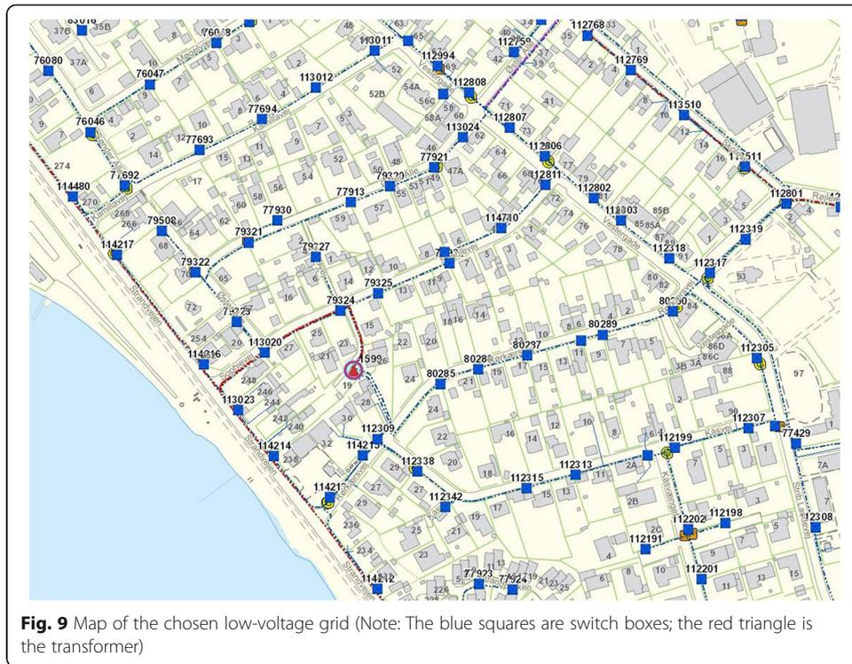
case study is to establish an agent-based simulation model for studying the impact of EV charging on grid stability in the low-voltage distribution grid of a residential area where the number of EVs is expected to increase towards 2030.
