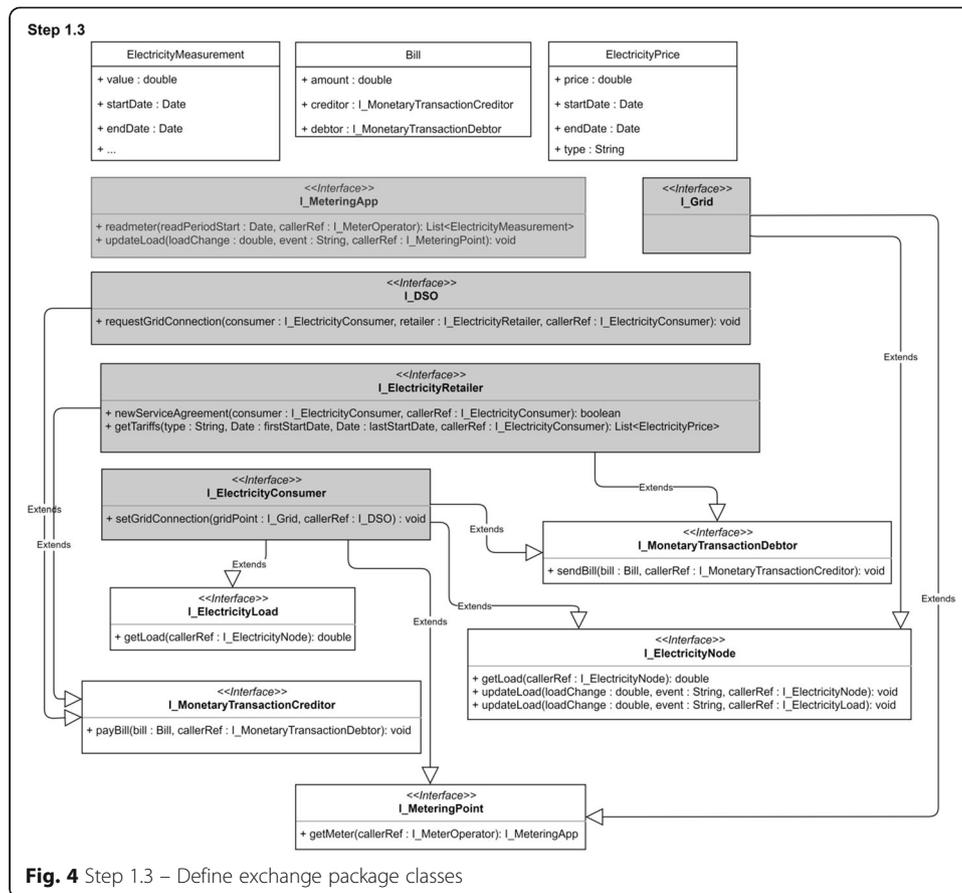
interface might feature multiple versions of the same method with different caller-Ref argument types, e.g. the *I\_ElectricityConsumer updateLoad* methods in Fig. 2. The number of versions can be reduced by convening the calling interface types under a common super-interface that reflects their similarities. Creating generic role interfaces has the following purposes and potential contributions they can provide to ABM of energy systems:
