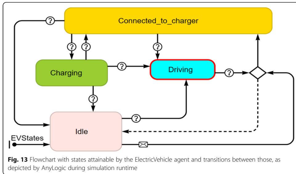
Upon the departure of a driving trip, the ElectricVehicle changes to the Driving state and upon arrival, the vehicle is immediately connected to the charger, hence changing to the Charging or Connected to Charger states, while the DomesticConsumer agent schedules the departure and arrival time of the next trip and sends this information to the Electric Vehicle agent.
