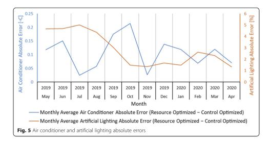
that the range for the luminosity is much wider than the temperature, with 0% to 100% and 18 °C to 28 °C, respectively. The maximum monthly average absolute error, for the artificial lighting luminosity, is 5.020%, and a minimum of 1.325%.
