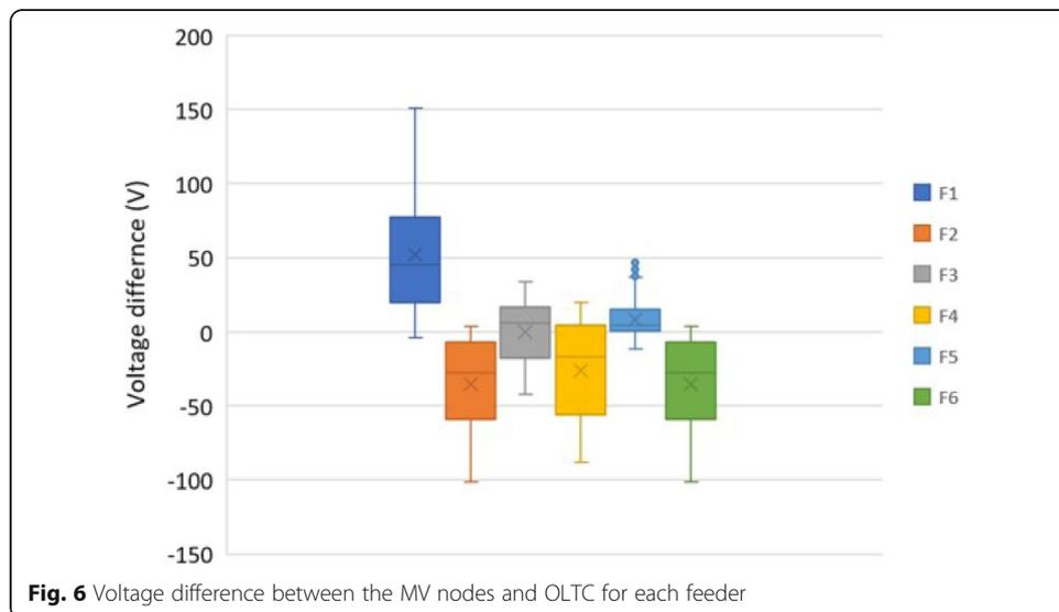
**Fig. 6** Voltage difference between the MV nodes and OLTC for each feeder
