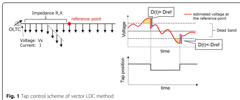
**Fig. 1** Tap control scheme of vector LDC method
