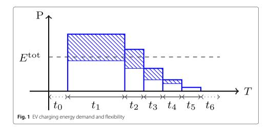
requesting energy over time, given the typical load curve of such a battery. While there is a large capacity for consuming more energy during  $t_1$ , the amount needed between  $t_2$  and  $t_5$  is decreasingly flexible. Figure 2 is a visualization of a forecast for the production of a given PV plant from a residential household.
