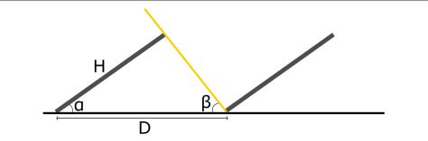
**Fig. 2** Distance D between two modules for a given module height H, tilt angle  $\alpha$  and solar elevation  $\beta$
