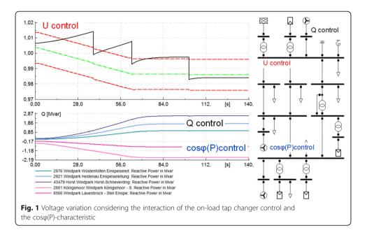
are set to control the voltage via providing or absorbing reactive power in the so called  $\cos\phi(P)$  control for decentralized energy resources.
