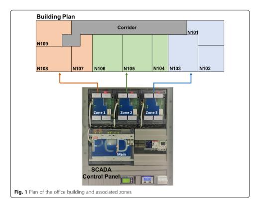
According to Fig. 1, the offices N101, N102, and N103 are belong to zone 1, N104 to N106 are dedicated for zone 2, and N107 to N109 are categorized in zone 3. Each zone contains one distributed PLC and one energy meter and a group of sensors.
