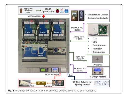
CO2, air quality, and illumination intensity) are connected to the related PLC in respective zone by 0–10 V Analog Input.
