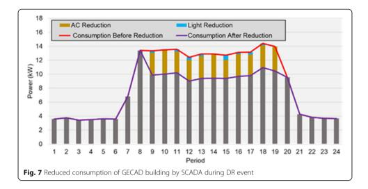
as Fig. 8 – (b) shows. Similar to ACs, the lights with low priority is reduced first. Then, the system reduced the high priority lights. Also, there are some periods during optimization, namely period #10, #14, and #19, the AC reduction attains to around 3.4 kW, and therefore, there is no reduction in the lighting system.
