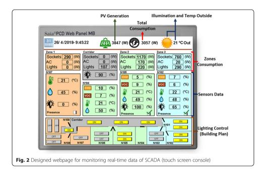
remote control of ACs, somehow the SCADA takes decision for each AC and transmits the desired command to each AC controller (Arduino\*) via Ethernet interface; Arduino controls the AC based on the SCADA decision (turn OFF/ON, and regulating the temperature) and fan for DR participation.
